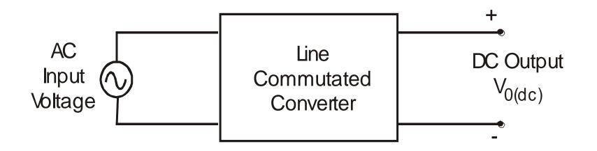
Type of input: Fixed voltage, fixed frequency ac power supply.
